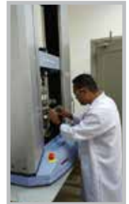
Tear & tongue strength test
